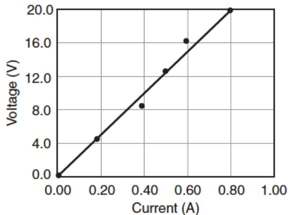
Using the graph, determine the resistance of the copper wire.
